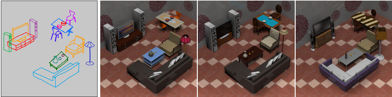
Figure 1: Without any user intervention, our framework automatically turns a freehand sketch drawing depicting multiple scene objects (left) to semantically valid, well arranged scenes of 3D models (right). (The ground and walls were manually added.)
